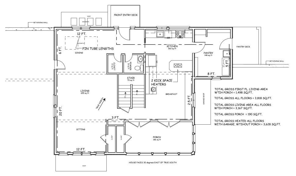
TOTAL LENGTH OF FIN TUBE RADIATION = 68.5 FT. + 2 KICK SPACE UNITS IN KITCHEN FIRST FLOOR LOOP IS 36.5 FT. OF HEAD AT 8 GPM. MANIFOLD TO MANIFOLD, DOES NOT INCLUDE BOILER
