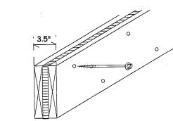
TYPICAL HEADER, PAIR OF 2x10's w/ 1/2" OF PLYWOOD, GLUED AND SCREWED. USE TIMBER TECH SCREWS, 1.5" FROM EDGES, 8" O.C., STAGGERED TOP & BOTTOM
